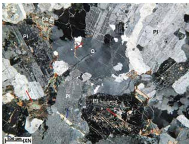
Figure 1. Mineralogy of gradiorite from XRD Red arrows: calcite, blue arrows: zeolite, pink arrow: chlorite.
